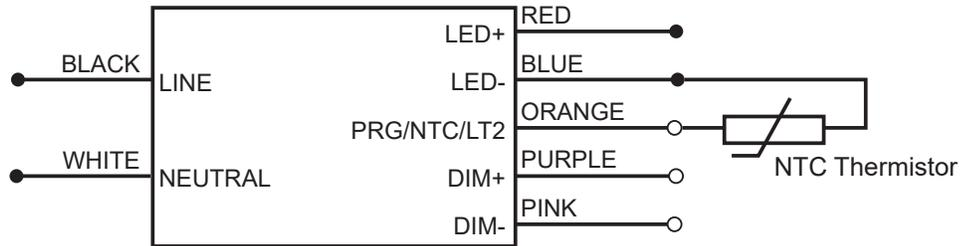
In the end application, care must be taken to place the NTC thermistor close to the hottest spot on the LED module. If LED thermal protection is not required the NTC port on the LED power supply connector can be left open.
