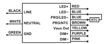
In the end application, care must be taken to place the NTC thermistor close to the hottest spot on the LED module. If LED thermal protection is not required the NTC port on the LED power supply connector can be left open. Vishay, EPCOS, Murata, Panasonic are some of the manufacturers of NTC thermistor. EPCOS part number for reference only - B57164K153J ( $15k\Omega$  @  $25^{\circ}C$ ). Murata part number for reference only - NCP03XH223J05RL ( $22k\Omega$  @  $25^{\circ}C$ ).
