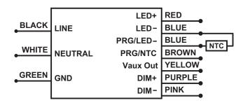
In the end application, care must be taken to place the NTC thermistor close to the hottest spot on the LED module. If LED thermal protection is not required the NTC port on the LED power supply connector can be left open. Vishay, EPCOS, Murata, Panasonic are some of the manufacturers of NTC thermistor. EPCOS part number for reference only - B57164K153J ( $15k\Omega$  @  $25^{\circ}C$ ). Murata part number for reference only - NCP03XH223J05RL ( $22k\Omega$  @  $25^{\circ}C$ ).
