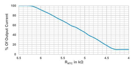
Derating start = 6.3kΩ; Derating end = 4.3kΩ; Min output level = 10%
