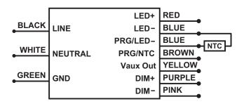
In the end application, care must be taken to place the NTC thermistor close to the hottest spot on the LED module. If LED thermal protection is not required the NTC port on the LED power supply connector can be left open. Vishay, EPCOS, Murata, Panasonic are some of the manufacturers of NTC thermistor. EPCOS part number for reference only - **B57164K153J (15kQ @ 25°C)**. Murata part number for reference only - **NCP03XH223J05RL (22kQ @ 25°C)**.
