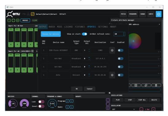
In the **Output** tab, click the **Scan for devices** button to search for any EMU Hardware connected to your computer. Once the device is detected, click the gear icon next to the device to access configuration options.
