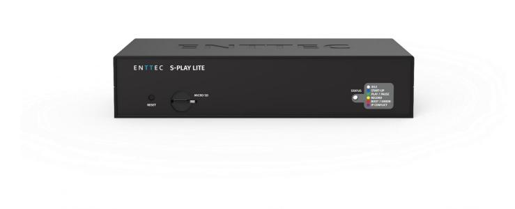
ENTTEC's S-PLAY LITE serves as a robust show recorder and playback controller, expertly integrating 3<sup>rd</sup> party system and external hardware for smart light show management.
