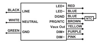
In the end application, care must be taken to place the NTC thermistor close to the hottest spot on the LED module. If LED thermal protection is not required the NTC port on the LED power supply connector can be left open. Vishay, EPCOS, Murata, Panasonic are some of the manufacturers of NTC thermistor. EPCOS part number for reference only **B57164K153J (15k\Omega @ 25°C)**. Murata part number for reference only - **NCP03XH223J05RL (22k\Omega @ 25°C)**
