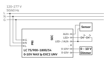
Class 2 Circuit, Suitable for Class 1 or Class 2 wiring only.
