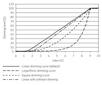
Dimming profiles programmable via NFC.
