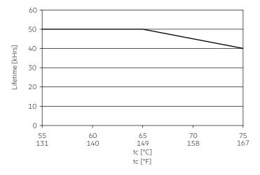
$The \ LED \ driver is designed for a life-time \ stated \ above \ under \ reference \ conditions \ and \ with \ a failure \ probability \ of less \ than \ 10 \ \%.$
