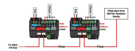
**Note:** When using CVC4s with any product within the Pixelator Family, set the P-Link port you have connected your CVC4s to output WS2812b with colour ordering RGB. This will convert your input DMX signal 1:1 into P-Link allowing you to mix and match CVC4 operating modes within the same String and patch them within your lighting control software.
